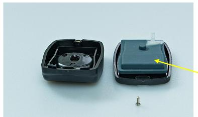
Lift membrane cover to expose battery.
