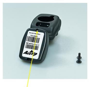
Remove screw, once removed turn over. Lift case from top and pull slightly forward.
