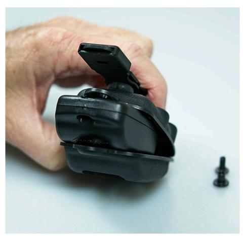
With case slightly open remote should drop from the back, place a finger in the front opening and gently push the remote free of the case.
