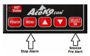
Alert will activate. During Pre alert Snooze can be manually reactivated (By pressing OK). Only 3 snooze periods are allowed.
